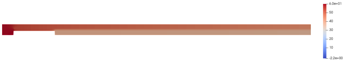
Figure 6.14: Pressure at DPF's inlet in Case 2.
