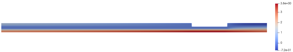
Figure 6.13: Horizontal velocity at DPF's outlet in Case 2.
