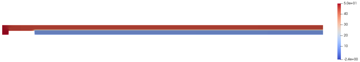
Figure 6.6: Pressure at DPF's inlet in Case 1.
