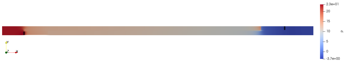
Figure A.18: Pressure at DPF in Case 4 obtained with Mesh 1.
