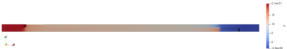
Figure 6.38: Pressure field plotted in the x_1 - x_3 plane.
