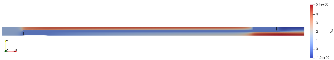
Figure A.17: Horizontal Velocity at DPF in Case 4 obtained with Mesh 1.
