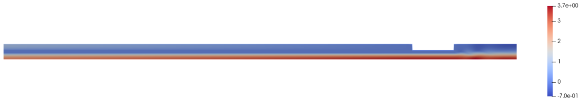
Figure 6.5: Horizontal velocity at DPF's outlet in Case 1.
