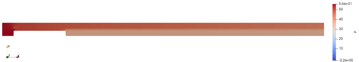
Figure A.7: Pressure at DPF's inlet in Case 2 using quadratic mesh.
