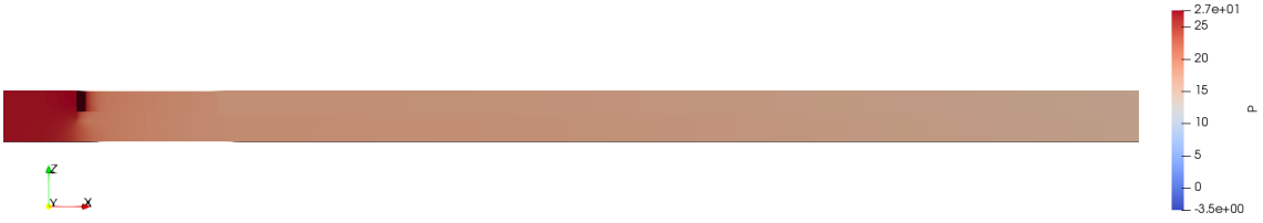
Figure 6.30: Pressure field at the DPF's inlet plotted in the x_1 - x_3 plane.
