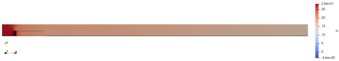
Figure A.15: Pressure at DPF's inlet in Case 3 obtained with Mesh 2.
