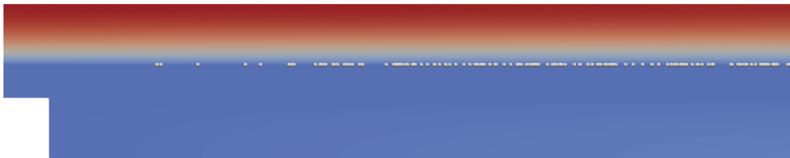
Figure 6.17: Horizontal velocity at DPF's inlet and particulates trapped in the porous wall at Case 2.
