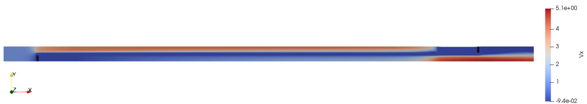
Figure A.19: Horizontal Velocity at DPF in Case 4 obtained with Mesh 2.
