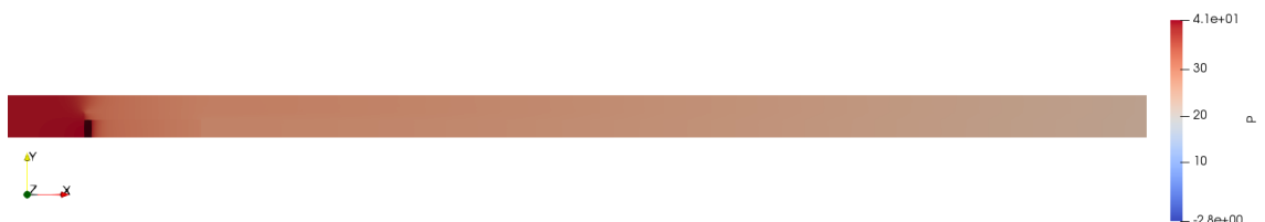
Figure A.11: Pressure at DPF's inlet in Case 3 obtained with Mesh 1.
