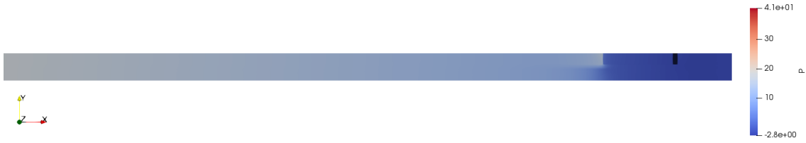
Figure A.12: Pressure at DPF's outlet in Case 3 obtained with Mesh 1.
