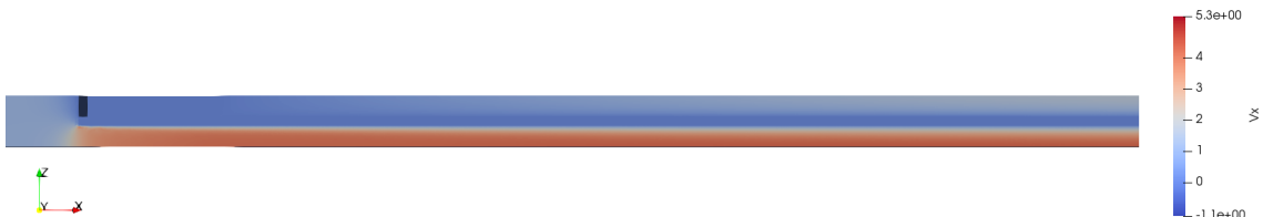
Figure 6.26: Horizontal velocity field at the DPF's inlet plotted in the x_1 - x_3 plane.
